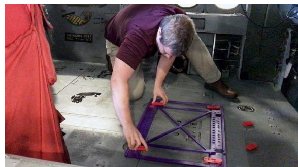
171026-N-JM744-002 (Patuxent River, MD) A member of the MH-60S Gunner Seat prototype team successfully installs the 3D printed floor mount in the Seahawk helicopter at Naval Air Station Patuxent River, Maryland, Oct. 26. (U.S. Navy photo)
